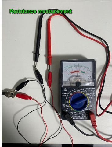
16, If the resistance is  $0\Omega$  or insulation in any range, the wire breakage on the Laue camera side may be considered.
